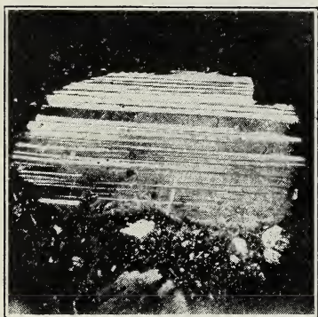
Figure 57. Photomicrograph of oligoclase, a sodium bearing feldspar, showing the composite character of some minerals. Courtesy Prof. A. N. Winchell.
